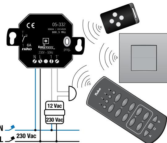
**! This product must be secured with a miniature circuit breaker (MCB) of max. 6 A in the electrical cabinet. The MCB rating is limited by national installation rules.**
