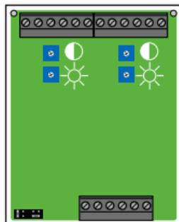
Output 1 can be adjusted by means of the 2 left potentiometers, output 2 by means of the right one.
