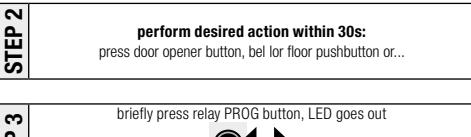
**Setting the relay output activation time between 0.5s and 128s (factory setting = 1s)**
