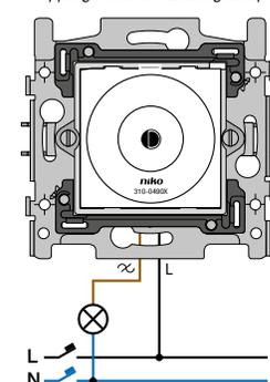
This product must be secured with a miniature circuit breaker (MCB) of max. 16 A in the electrical cabinet. The MCB rating is limited by national installation rules
