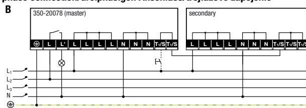
Monofasige aansluiting/connexion monophase/single phase connection/einphasigen Anschluss/jednofazove zapojenie
