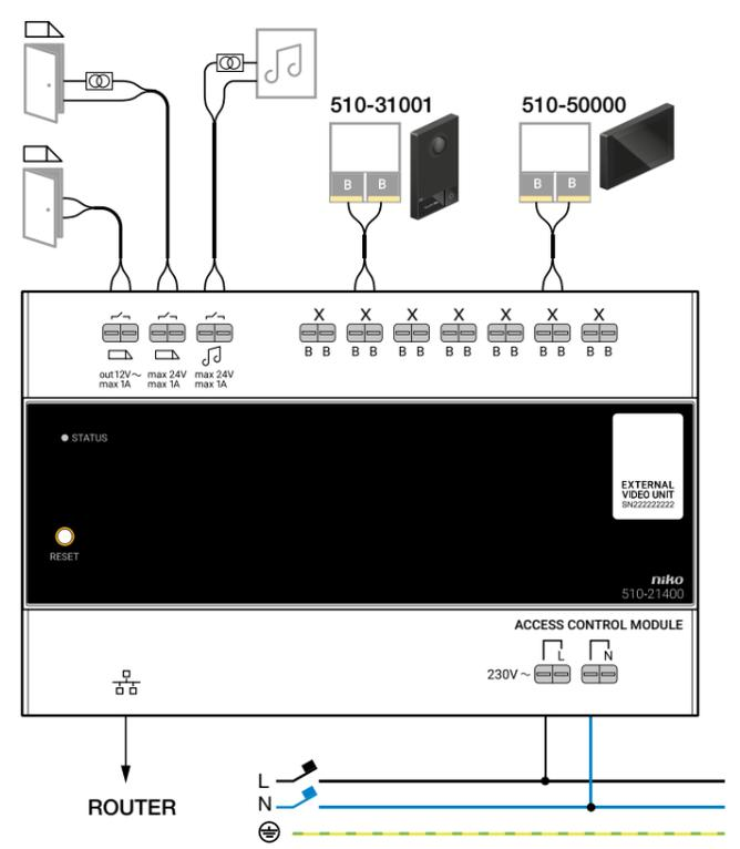
⚠ This product must be secured with a miniature circuit breaker (MCB) of max. 16 A in the electrical cabinet. The MCB rating is limited by national installation rules.
